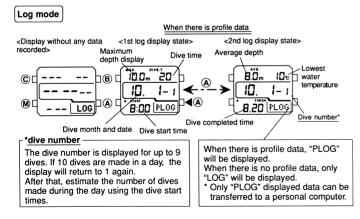
It separately displays both 1st log display and 2nd log display; you can select by pressing A button 1st log display......Maximum depth, dive time, dive month and date, dive number, dive start time 2nd log display.....Average depth, lowest water temperature
